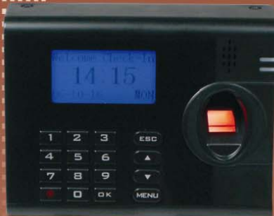
Finger Print access controller with USB port and UrU sensor
